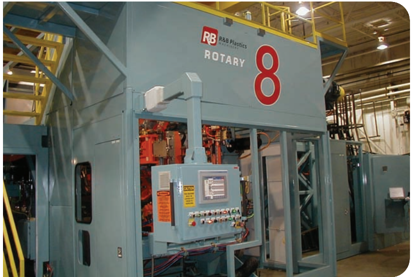
R & B works with Rockwell Automation to offer users scalable solutions for parison-control retrofits. This approach leaves all other machine control systems in place.
